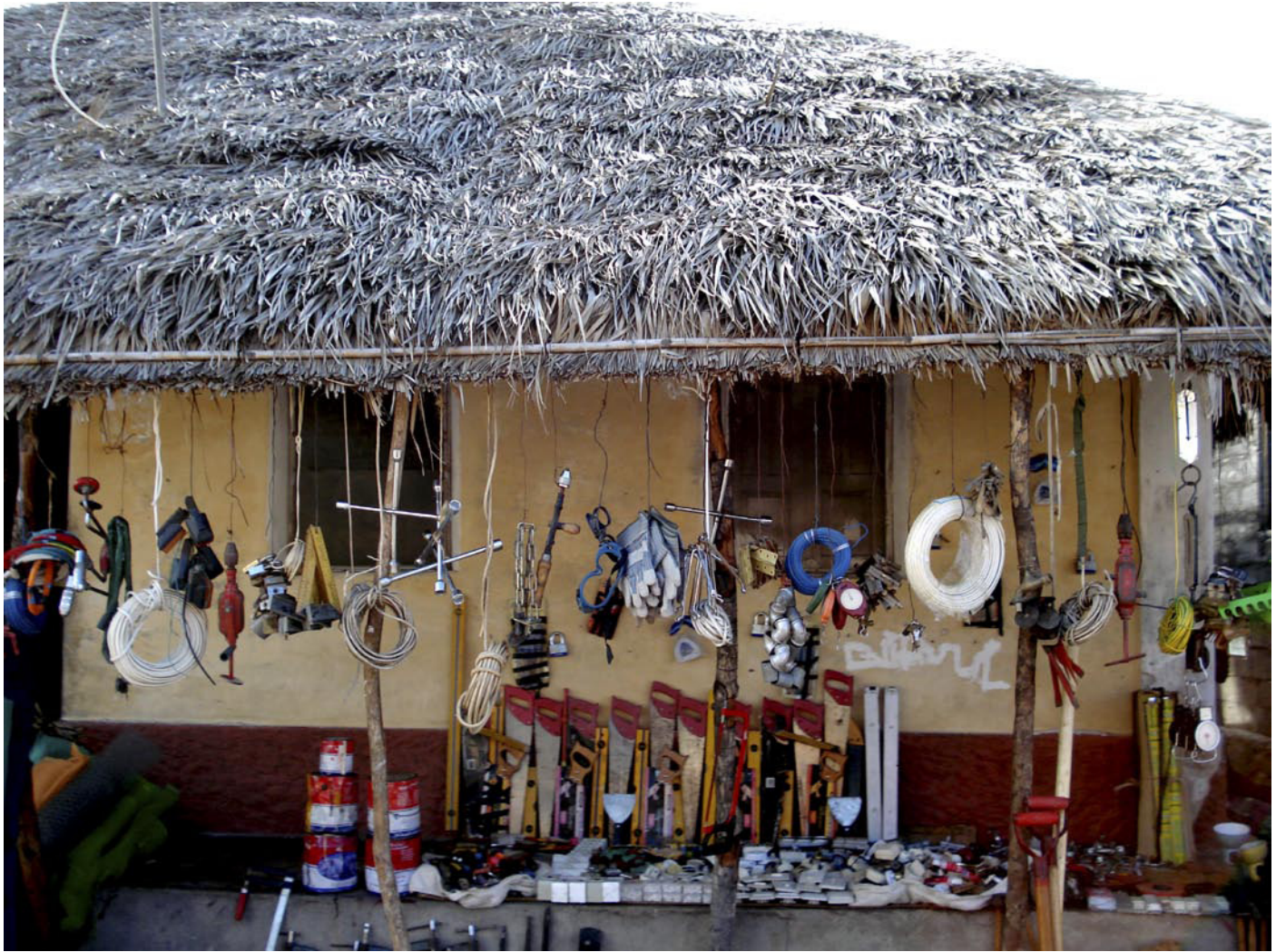
Figure 2. Vernacular urban housing in Mozambique, with veranda serving as shop, which illustrates both mixed “traditional” construction (palm thatch of the roof) and modernised vernacular (walls/openings), as well as use of “traditional” space (overhung veranda) for modern activity - small-scale “informal” commerce. (Source: Paul Jenkins)-
