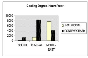
**Figure 7**: Comparison of the intensity of overheating in a Contemporary house and Traditional houses from different climatic zones in Thailand (Source: Authors)
