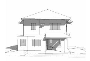
**Figure 9**: Inadequate shading on west façade of a contemporary house in the central region at 3pm in June (Source: Antarikananda, 2005)
