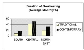
**Figure 6**: Comparison of the duration of overheating in a Contemporary house and Traditional houses from different climatic zones in Thailand (Source: authors)
